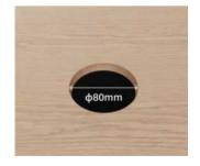
Make a cutout of diameter Ø80mm on the desired surface.
